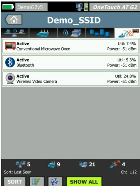
Figure 25: Unique Interferer analysis classifies sources of non-802.11.
