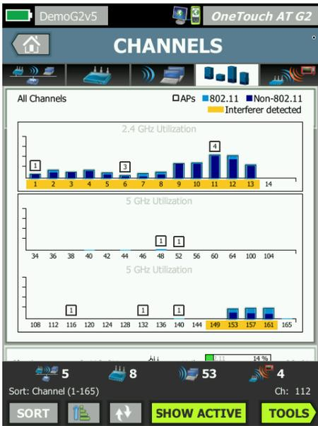
Figure 23: Analyze Wi-Fi health by each available channel.
