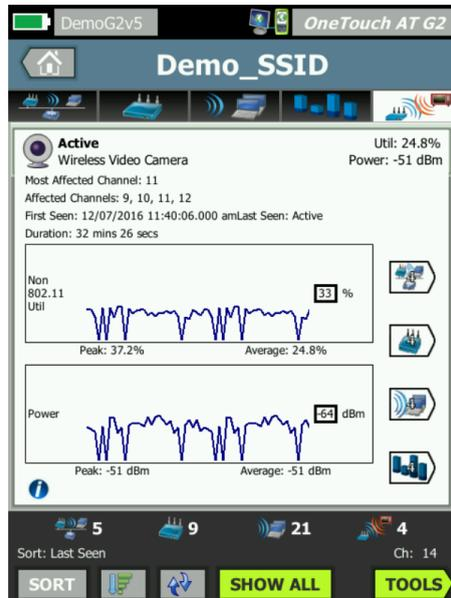
Figure 26: Detailed information about a specific interference source.
