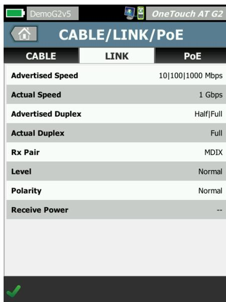
The screenshot shows the OneTouch AT G2 interface with the 'CABLE/LINK/PoE' test results. The interface has a status bar at the top with 'DemoG2v5' and 'OneTouch AT G2'. Below the title bar, there are three tabs: 'CABLE', 'LINK', and 'PoE'. The 'LINK' tab is selected. The results are displayed in a table format with a green checkmark at the bottom left.
