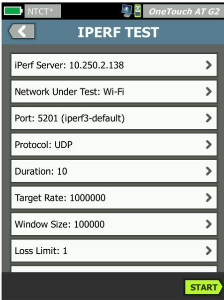
Figure 21: Setup for TCP Window Size and Threshold.
