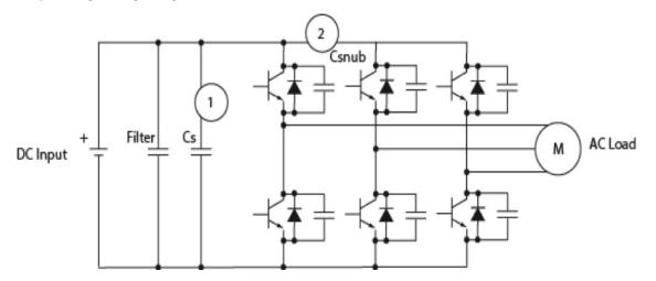
Figure 1. Circuits exposed to increased voltages, such as the DC-Link and snubber, need to be constructed with the voltage rating of the capacitors in mind.
