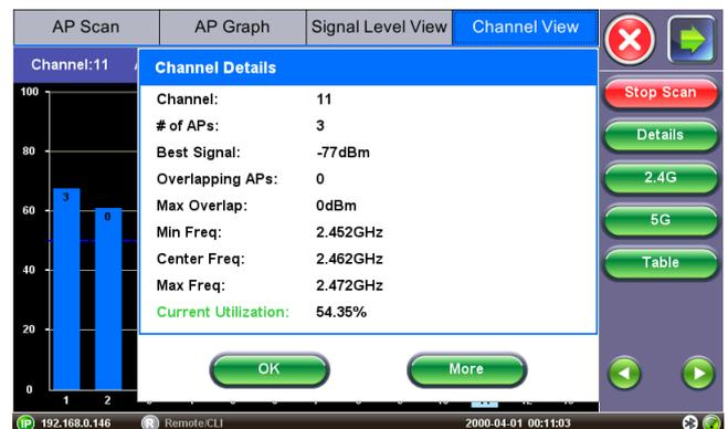
Detailed channel measurements can be sorted by any field including utilization %, number of APs, number of co-channel APs and strongest signal. This information is crucial as technicians need to identify if performance issues are linked to high channel utilization and must quickly decide if reconfiguring the AP to a new channel is advisable.
