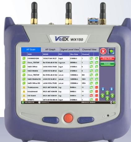
The WX150 test set is a compact and lightweight addition to the WiFi Air Expert family. It provides all the tools necessary for WiFi networks discovery, survey, optimization, performance testing and troubleshooting in a compact form factor.
