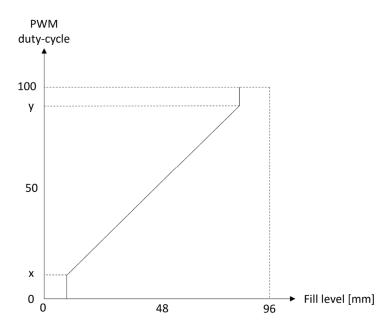
When fill level exceeds the active sensing area, the mapping function will get non-linear.
