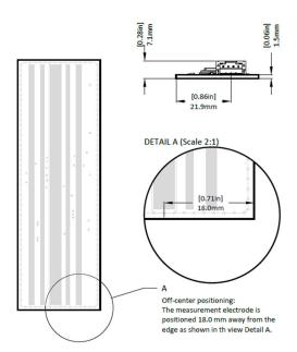
The active sensing area of the sensor is on the bottom side of the PCBA. To avoid influences on the capacitive measurement system, keep area free of metallic surfaces or mounting components e.g. metal screws (> 5 mm distance to the outer bounds of the active sensing area).
