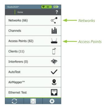
2) From the Networks screen use the touchscreen to select the SSID on which you want to run the performance test. If you decided to use the Access Points option, then you need to select an access point.
