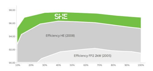
including cost of ownership, particularly in markets where power prices are above average. Backwards compatibility with all 3kW Flatpack2 modules makes upgrading simple - modules can be hot-swapped without interfering with system operation.
