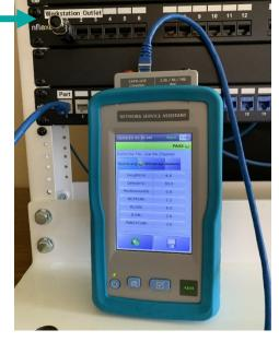
The main test unit of NSA is similar to a main unit of AEM's award-winning certification tester, TestPro that comes in a pair for dual-ended testing. Because the NSA performs a single-ended cable test, it comes with a small passive termination plug called *NSA Remote*, at the remote end, which helps to significantly reduce the overall cost of the test equipment while providing an ANSI/TIA 1152-A complaint cable test.
