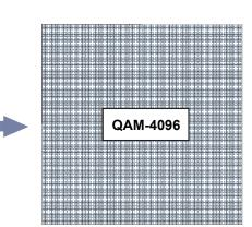
• Dynamic adaptation to line conditions. When an impairment appears, the affected OFDM subcarrier can downshift to a lower order modulation to help ensure robust, error free transmission
