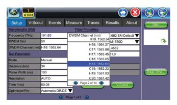
**CWDM** – All 18 wavelengths defined in ITU G.694.2 grid are selectable via pull down menu.
