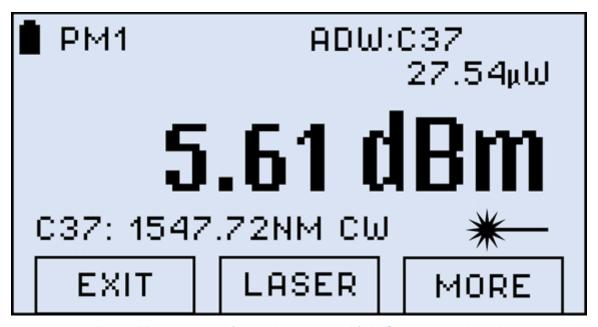
Power Meter channel is set the same as Light Source wavelength
