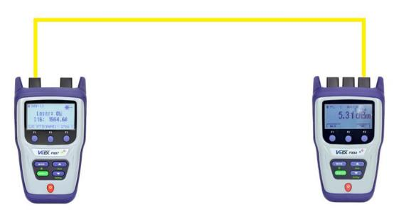
FX87 connected over fiber under test to FX-8x OPM
