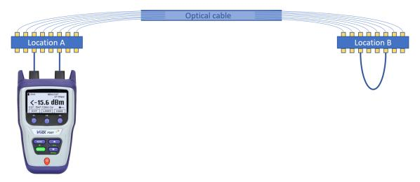
Using one device for optical power measurement (Loopback function)
