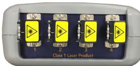
**OLS ports:** Used to provide 4 independent, continuous light sources at the specified wavelengths. Pairing the OLS with an OPM allows you to test for loss or end-to-end continuity on a CWDM network.
