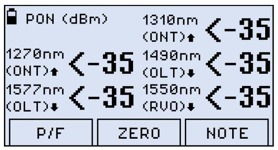
PON Burst mode measurement results as values, FX81
