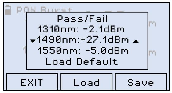
Setting Pass/Fail thresholds, FX80
