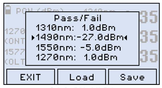
Setting Pass/Fail thresholds, FX81
