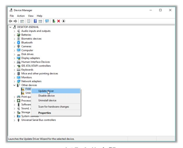
Installing the driver for FX8x
