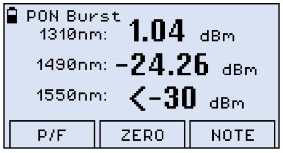
PON Burst mode measurement results as values, FX80
