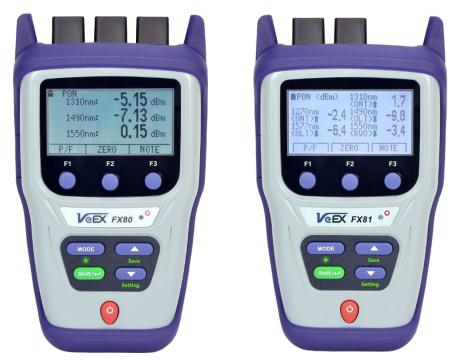
FX80/FX81 front view: FX80 with opt BB-OPM on left, FX81 5-wavelength version on the right
