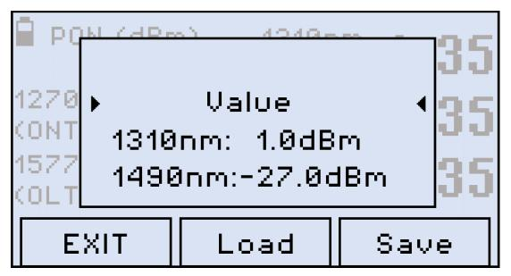
Switching from thresholds to values for the same measurement, FX81
