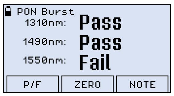
PON Burst mode measurement results as P/F thresholds, FX80
