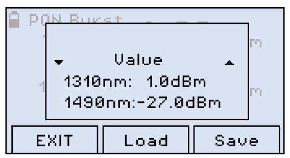
Switching from thresholds to values for the same measurement, FX80
