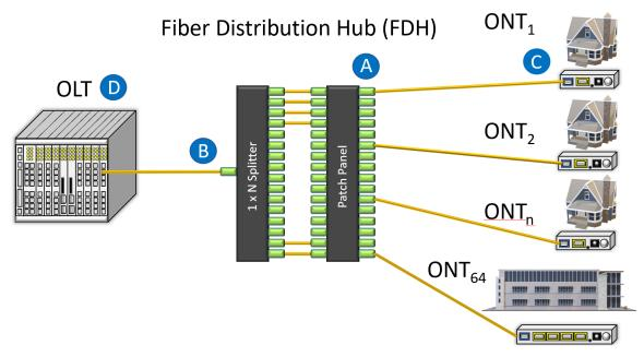
A typical passive optical network (PON) with possible points of measurement
