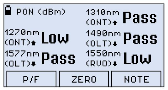
PON Burst mode measurement results as P/F thresholds, FX81
