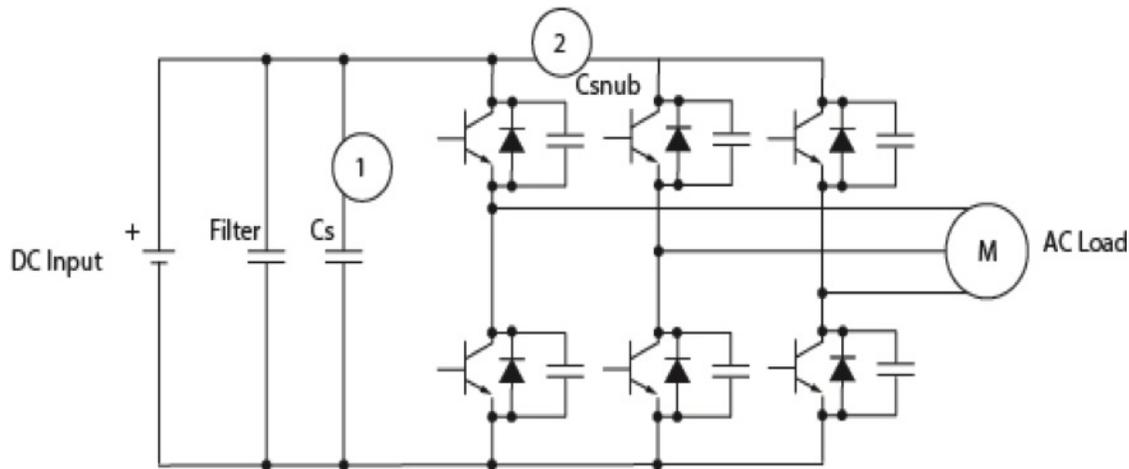
*Figure 1. Circuits exposed to increased voltages, such as the DC-Link and snubber, need to be constructed with the voltage rating of the capacitors in mind.*
