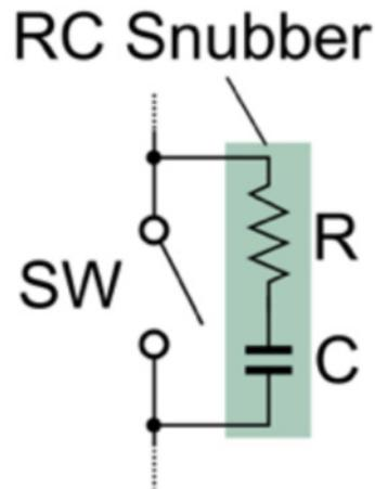
Figure 3. A depiction of a basic snubber circuit. (Source: [Wikipedia](#))
