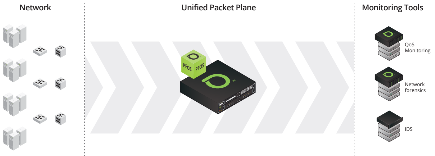
Figure 1: The NETSCOUT unified packet plane powered by PFOS (Packet Flow Operating System) logically separates the network from the monitoring systems.
